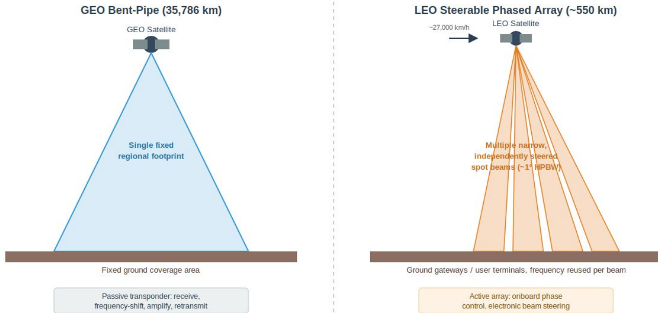
Fig. 1 — A bent-pipe GEO satellite illuminates one static footprint; a LEO phased array reforms several narrow, steerable beams every few microseconds.
